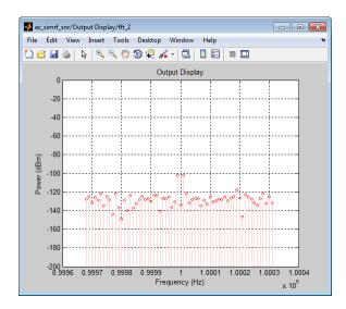
The measured PSD of -102 dBm/Hz for each tone is consistent with the 40-dB combined gain of the amplifier and mixer. The noise PSD in the figure is shown to be approximately 50 dB higher at the output, due to the gain and noise figure of the system.
