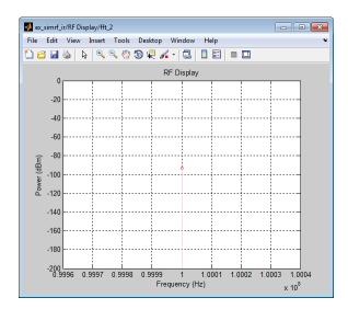
The modulation of the RF carrier is a constant envelope generated by a Continuous Wave block which generates a single peak centered at the carrier.
