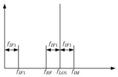
The preceding figure illustrates two input signals at the carriers  $f_{RF}$  and  $f_{IM}$  that both differ from the LO frequency,  $f_{LO1}$ , by an amount  $f_{IF1}$ . Mixing translates both input signals down to  $f_{IF1}$ . Perfect image rejection in the final stage of the receiver removes the image signal from the output entirely.
