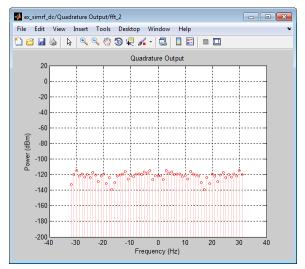
The quadrature output only contains noise because the input signal and blocker have no quadrature components.
