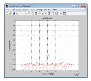
The measured power of each tone is consistent with the expected power level of a  $0.1-\mu V$  two-tone envelope:
