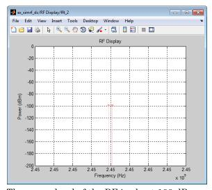
The power level of the RF is about 100 dBm.
