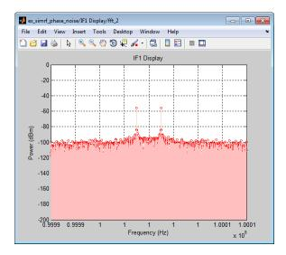
The figure shows that the LO phase noise has been transferred to the image. The RF signal on the carrier  $f_{I\!F\!1}$  is not visible in the figure because its power level is below the phase noise power of the downconverted image signal. The two visible peaks are at the same power as the IF shown in the previous section, "Create a Model with RF Interference" on page 2-2.
