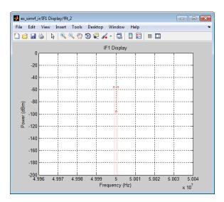
Both the RF and image appear on the carrier. The power level of the image 40 dB higher than the RF.
