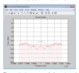
The quantization error exceeds the receiver noise.
